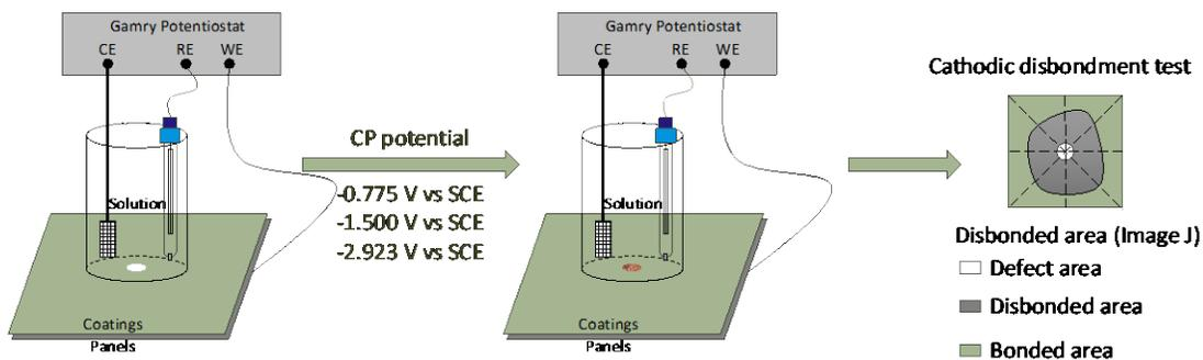
**Figure 6.** Coating cathodic disbondment testing procedure.
