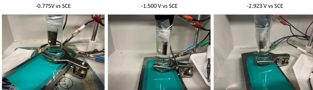
**Figure 7.** Cathodic disbondment testing of the liquid epoxy coating under different CP potential conditions of -0.775 V, -1.500 V, and -2.923 V vs SCE.
