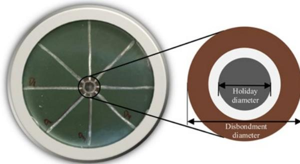
**Figure 10.** Representation of the area affected by CD in a coating exposed to CP.
