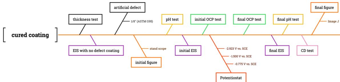
**Figure 5.** Experimental protocol for the study of coating cathodic disbondment.
