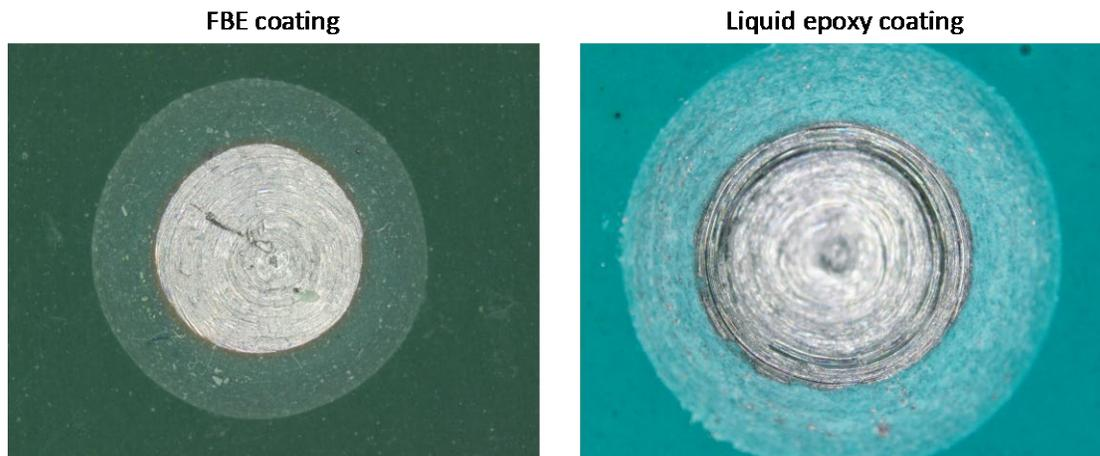
**Figure 3.** Coating samples with an artificial hole of FBE coating and liquid epoxy coating.
