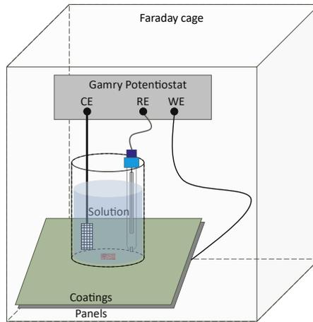
**Figure 4.** The electrochemical cell for the coating cathodic disbondment test. S type Q-panel as working electrode (WE), saturated calomel electrode as reference electrode (RE), and platinum sheet as counter electrode (CE).
