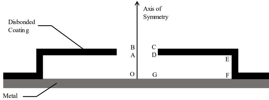
**Figure 9.** Schematic diagram of the simulation domain.
