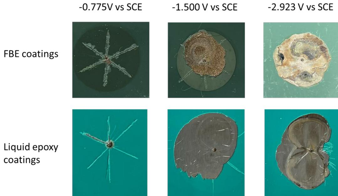
**Figure 8.** Cathodic disbondment test results of FBE coatings and liquid epoxy coatings under different CP potential conditions of -0.775 V, -1.500 V, and -2.923 V vs SCE.
