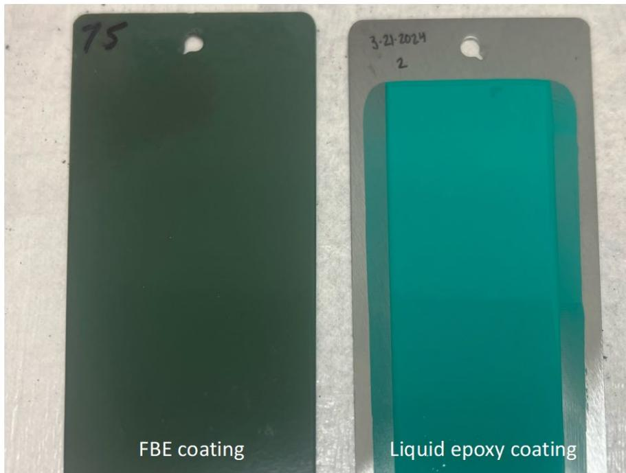
**Figure 2.** Perfect coating samples of FBE coating and liquid epoxy coating.
